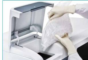
Special RV array design allows for accurate reaction vessel placement and avoids potential blockage.
