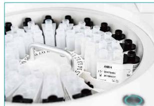
Non-contact vortex mixer design avoids liquid touching and eliminates the chance of cross contamination.
